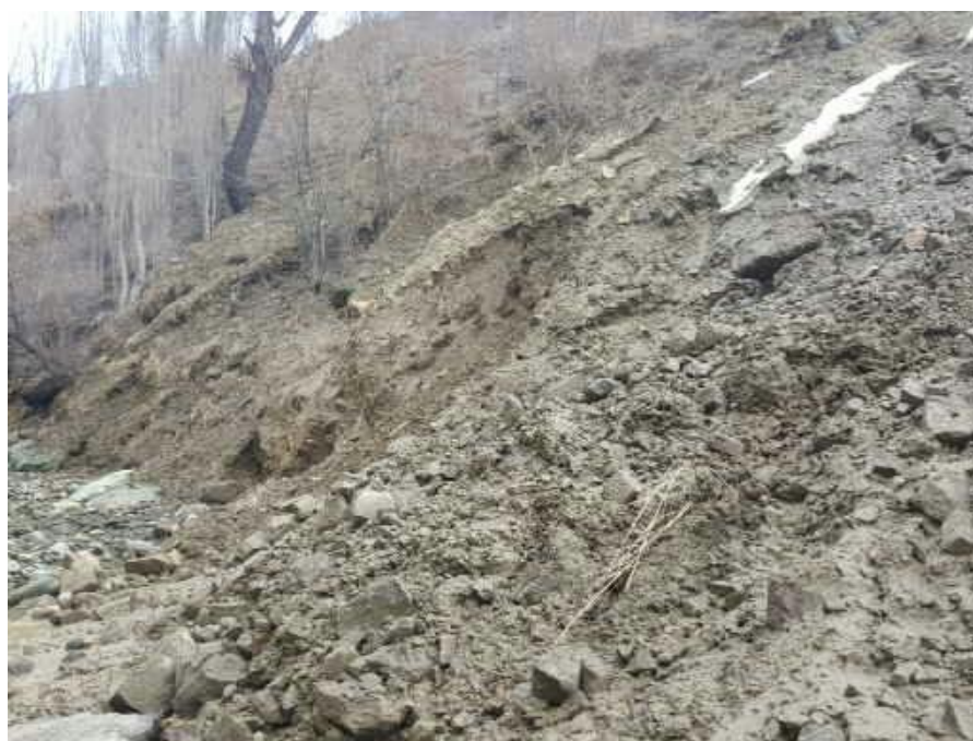
Figure 1 Weathered, shattered and jointed loose strata with high slope
